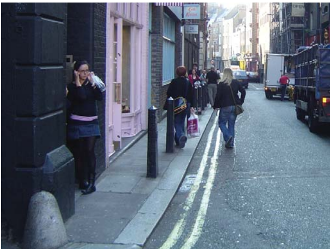
Shelton Street - Bollards line narrow footways, creating a pedestrian obstruction, pedestrians often having to resort to using the highway to avoid bollards and other pedestrians.
