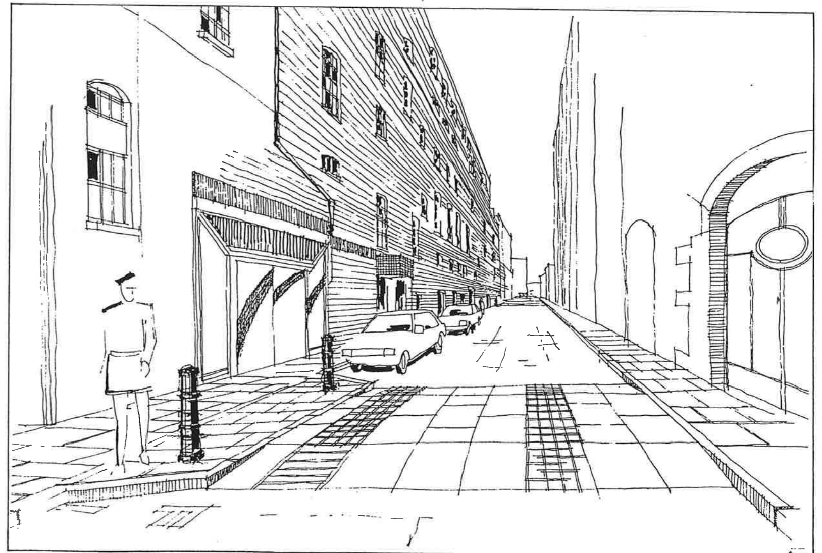
SKETCH VIEW OF A PROPOSAL FOR A SPEED HUMP IN EARLHAM STREET Note street furniture, like bollards, lamp columns etc should be in coordinated groups which relate to street features
