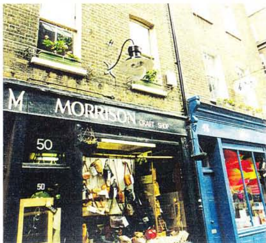
Example of a building fixed bracket lamp (left) to illuminate the highway in Neal Street, allowing the removal of the clutter of street columns.
