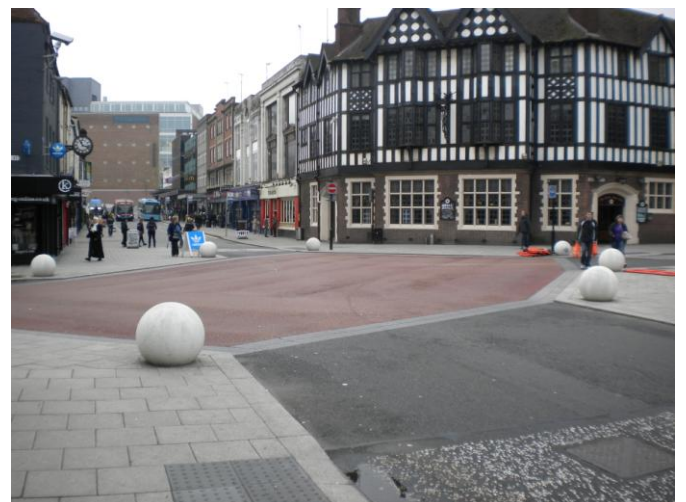
'Mastertint' coloured asphalt defines an atypical junction arrangement in Coventry
